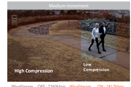
WiseStream OFF : 7260kbps WiseStream ON : 1817kbps
